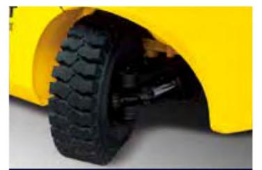
**Fully hydrostatic power steering**
