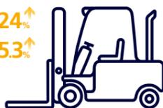
Maximum travel speed and drawbar pull are increased by 24% and 5.3%, respectively, by resetting rpm in the high-speed region of the engine and applying the gear of new transmission and drive axle of Hyundai Core Motion.
