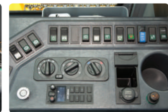
Centralized Instrument switch Panel
