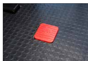
New floor mat & Dead man switch
